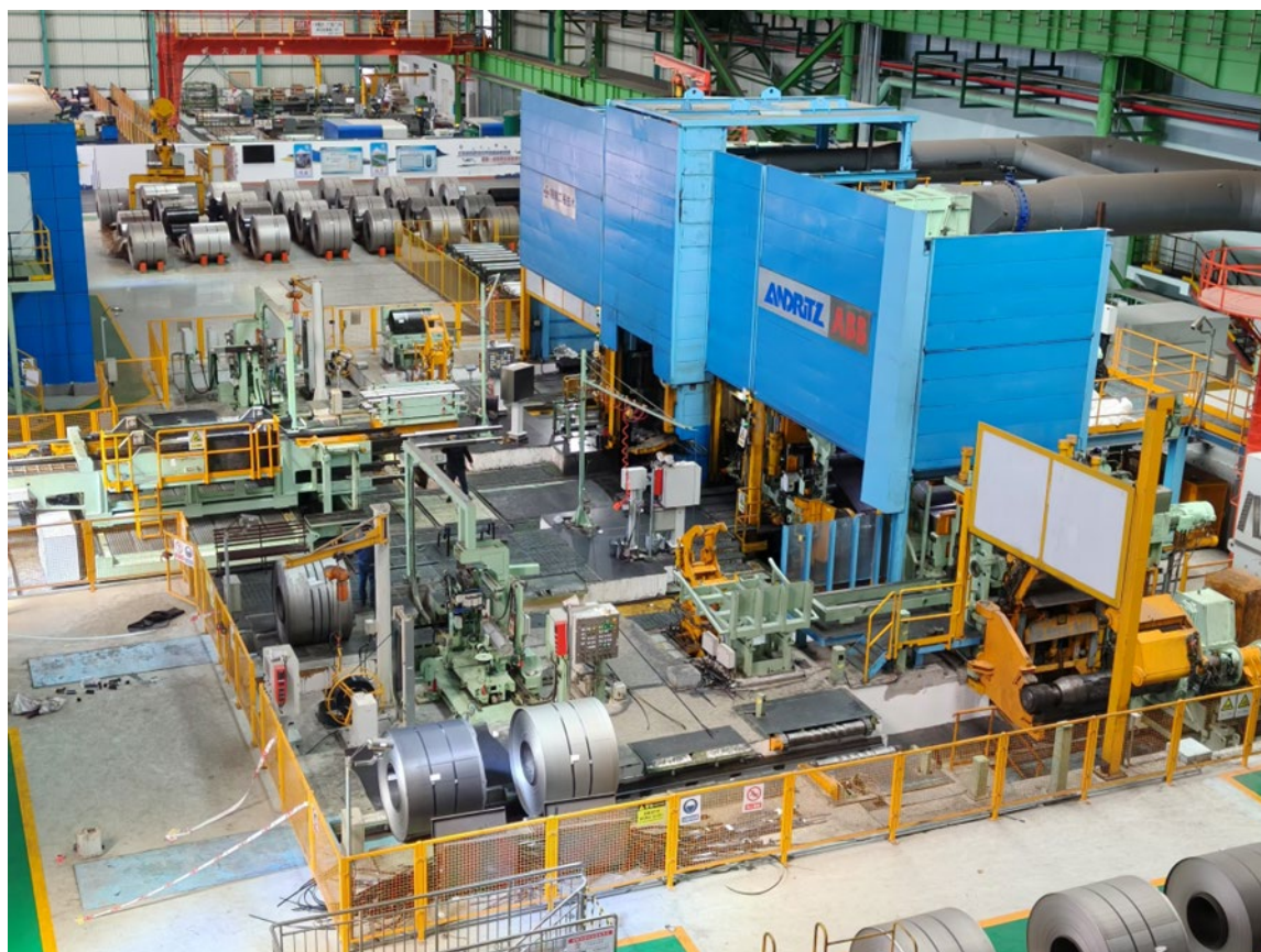
ANDRITZ's S6-high cold rolling mill at Xichang site
